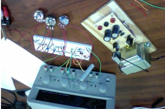
Figure 4. Analog circuit for the microphone and the pre-amplifier
